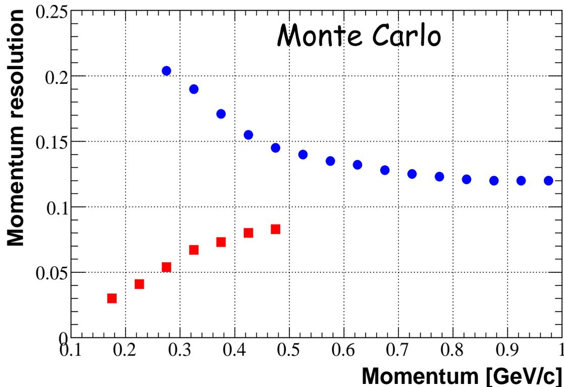
Blue - accuracy of momentum reconstruction by bending in the magnetic field
