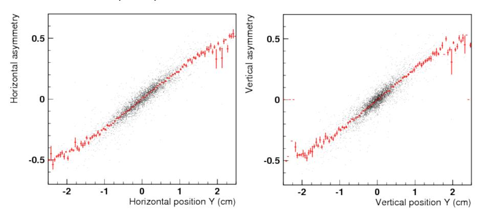
Asymmetry  $\eta$  in PMT signal correlated to position on calorimeter
