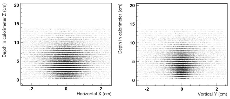
• Compton centering important, to avoid losing part of the shower (beam sizes from HERA used in this Monte Carlo simulation)
