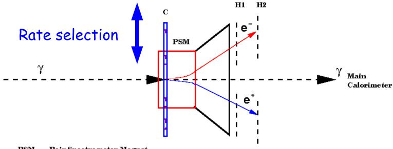
PSM -- Pair Spectrometer Magnet
