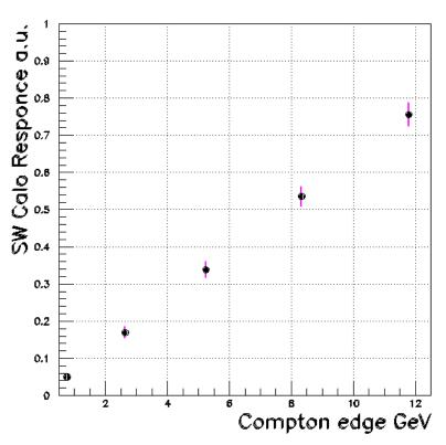
Use Compton edge to calibrate calorimeter
