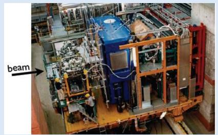
Polarized hydrogen (Long., Trans.), deuterium (Long.) Polarization flipped at 60-180 s time interval Unpolarized *H*, *D*, *He*, *N*, *Ne*, *Kr*, *Xe*
