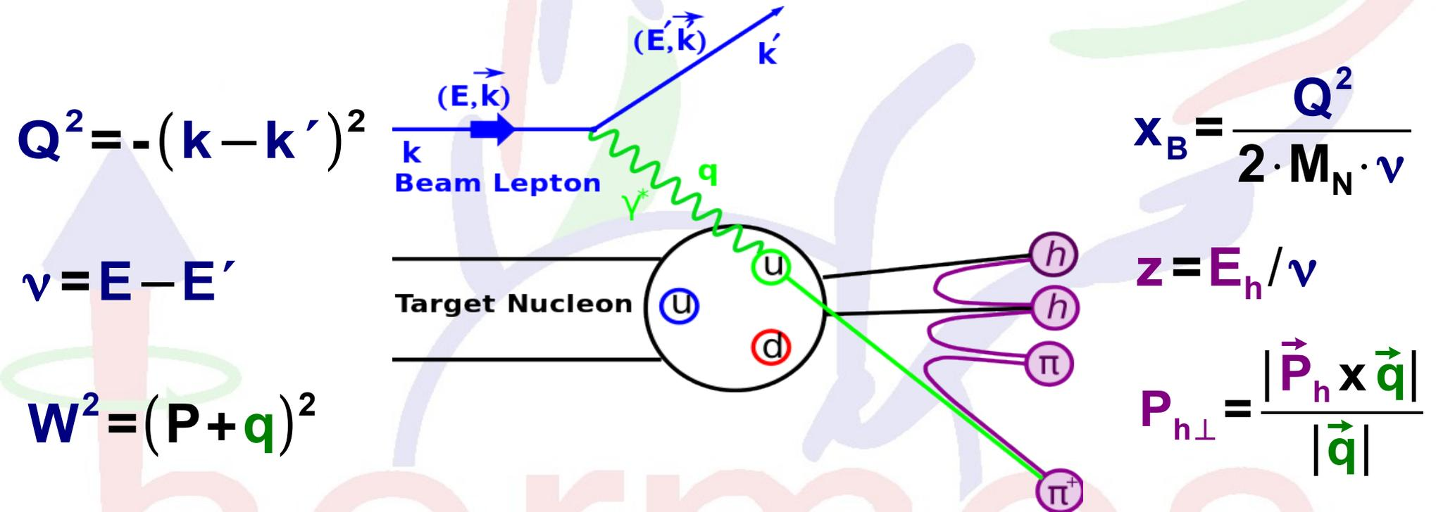
$$\sigma_{eN \rightarrow ehX} \sim \sum_q e_q^2 f_q(x_B, Q^2, \mathbf{k}_\perp^2) \sigma^{eq \rightarrow eq} D_q^h(z, Q^2, \mathbf{p}_\perp^2)$$
