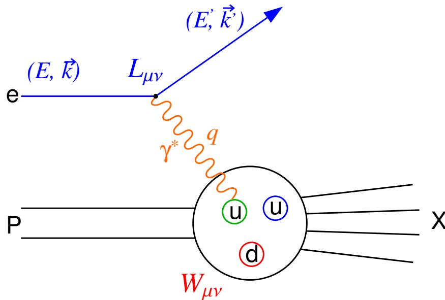
$$\begin{aligned} Q^2 &= -q^2 = -(k - k')^2 \\ \nu &\stackrel{\text{lab}}{=} E - E' \\ x &= \frac{Q^2}{2M\nu} \\ y &= \frac{\nu}{E} \end{aligned}$$
