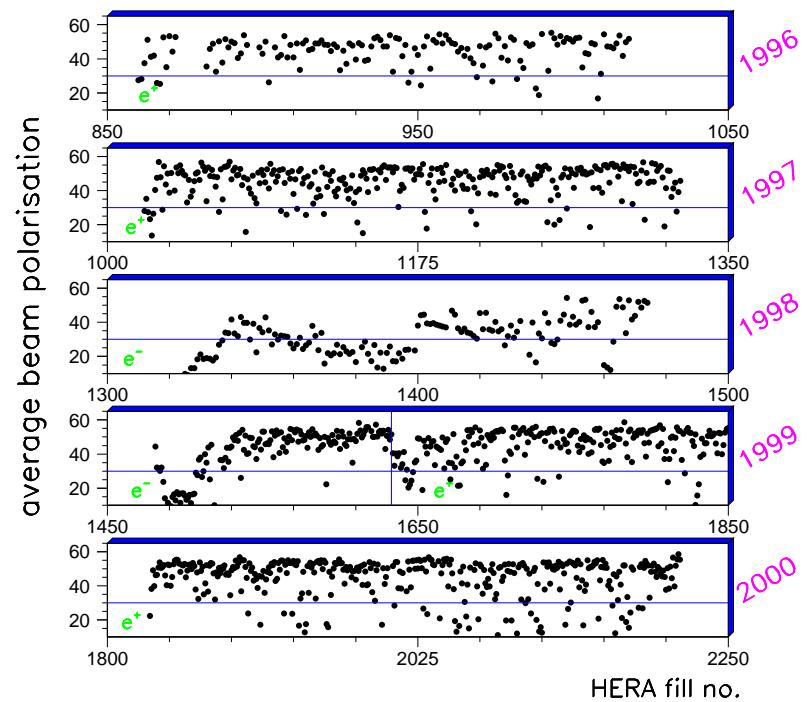
HERA-e beam self-polarized due to emission of synchrotron radiation
