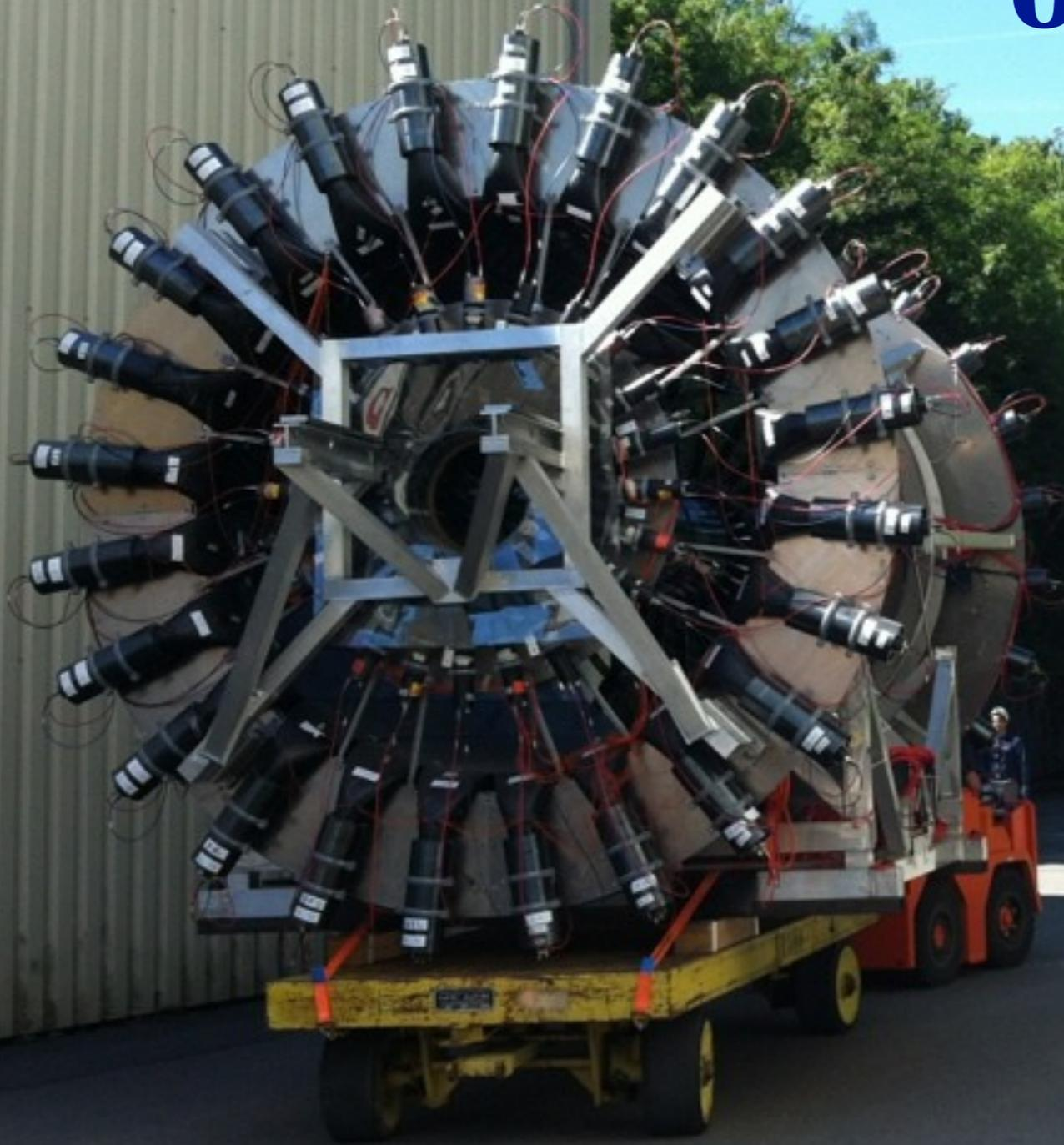
Preparing upgrade of CAMERA recoil proton detector: replace scintillators of inner ring to achieve better attenuation length (2015).
