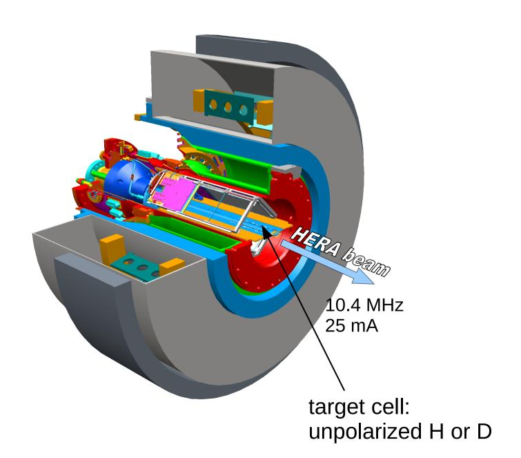
1 Tesla superconducting solenoid HERA BORDIN 10.4 MHz 25 mA target cell: 8 unpolarized H or D
