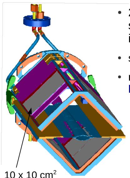
2 layers of double-sided silicon micro-strip sensors in beam vacuum
