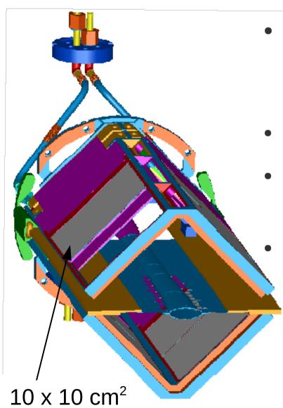
2 layers of double-sided silicon micro-strip sensors in beam vacuum
