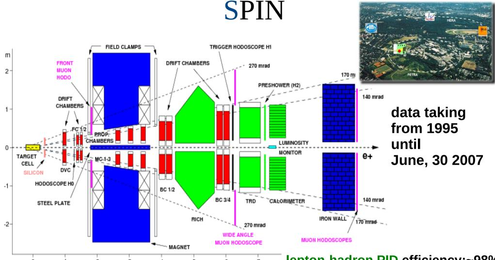
Beam longitudinally pol. e<sup>+</sup> & e<sup>-</sup> E= 27.6 GeV Gaseous internal target longitudinally pol. H,D,He transversely pol. H unpol. H,D,Ne,Kr,.. lepton-hadron PID efficiency:~98% hadron PID: RICH 2-15 GeV/c
