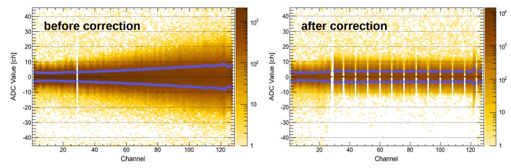
after common mode noise correction (based on 32 first channels of chip), increase of pedestal width with strip number
