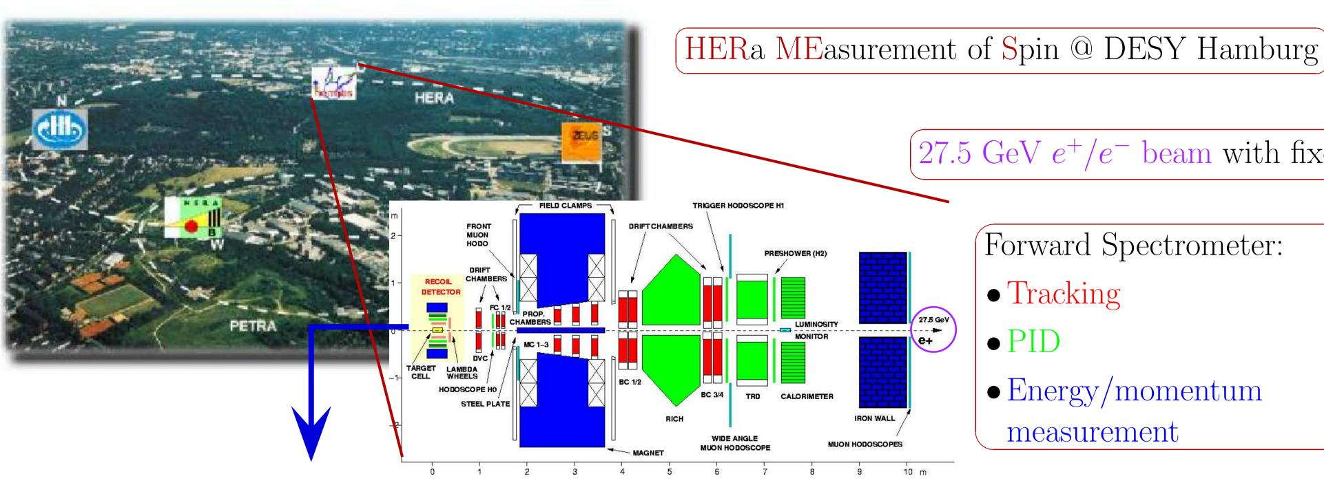
27.5 GeV  $e^+/e^-$  beam with fixed target (p-gas)
