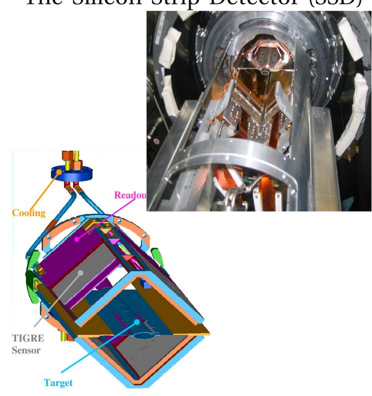
The SSD consisted of 8 modules of 2 double-sided silicon strip detectors (TIGRE) arranged in two layers around the target cell. It was used for position and energy measurement and identification of low momentum protons (125-450 MeV/c).
