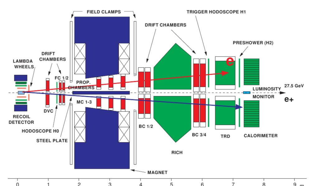
The HERMES spectrometer is a fixed target experiment and collected data on inclusive and semi-inclusive deep inelastic scattering of polarised positrons and electrons (beam momentum of 27.6 GeV/c and up to 65% beam polarisation) with polarised or unpolarised targets of H, D, and heavier targets. These data provide information on the spin structure of the nucleon.
