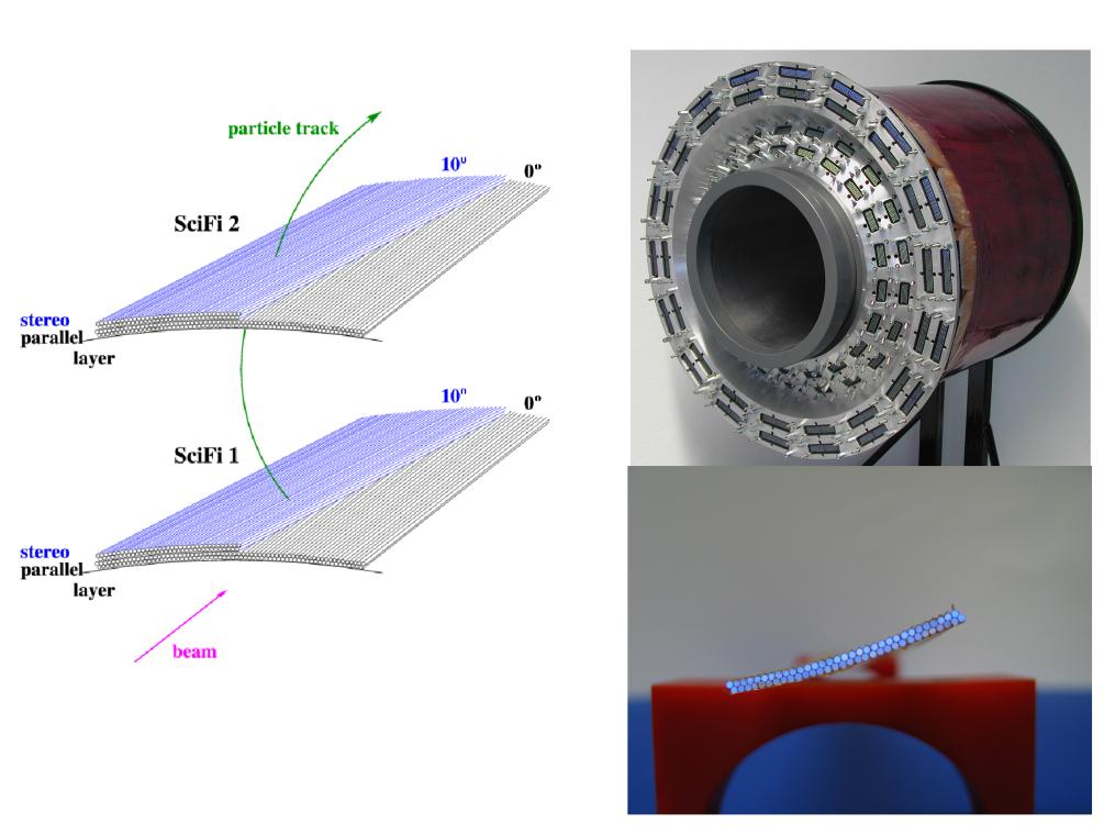
The SFT consisted of 2 barrels each with 4 layers of scintillating fibres. Each barrel had 2 parallel and 2 stereo layers for space point reconstruction.
