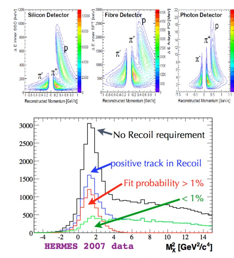
To select a clean sample of pure elastic events  $(ep\rightarrow ep)$  it is necessary to suppress the background of associated processes like  $ep\rightarrow e\Delta^+$  with  $\Delta^+\rightarrow p\pi^0$ . For this purpose the precise measurement of the recoiling particles is essential. The particle identification from the recoil data makes it possible to distinguish between pions and protons.
