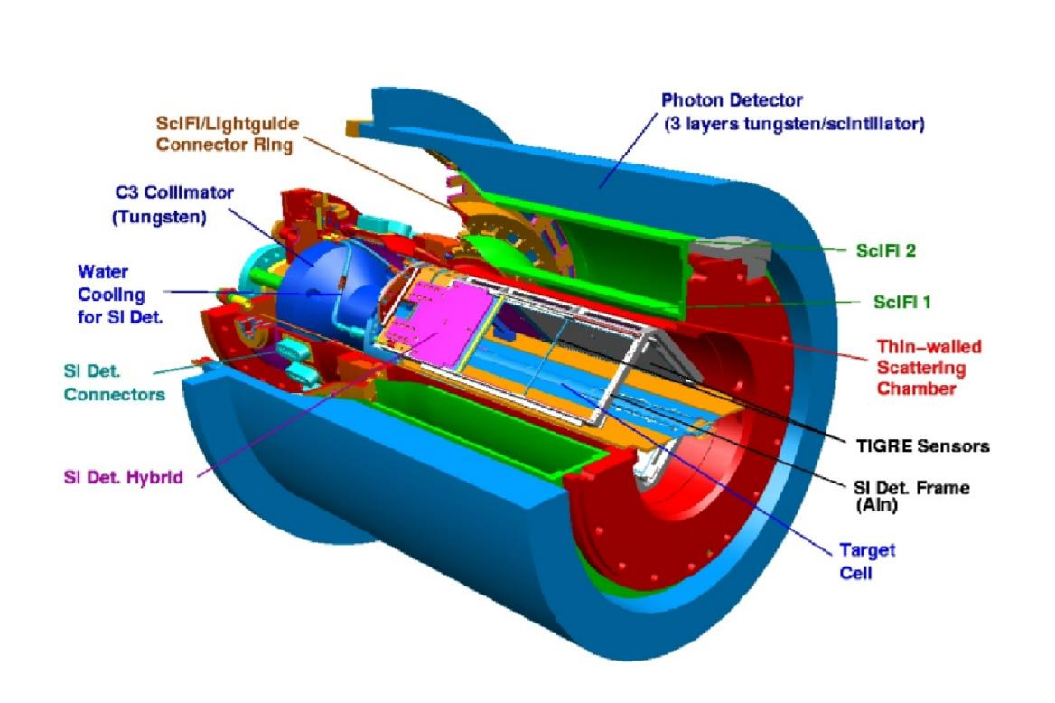
The Recoil Detector can detect recoiling protons (125-400MeV/c), improves (Mandelstam) t-resolution and suppress the background. It consists of a Silicon Strip Detector (SSD), a Scintillating Fibre Tracker (SFT) and a Photon Detector (PD). A solenoid magnet provides a 1T longitudinal magnetic field for the measurement in the SFT and allowes to reduce the background from Møller electrons in the SSD.
