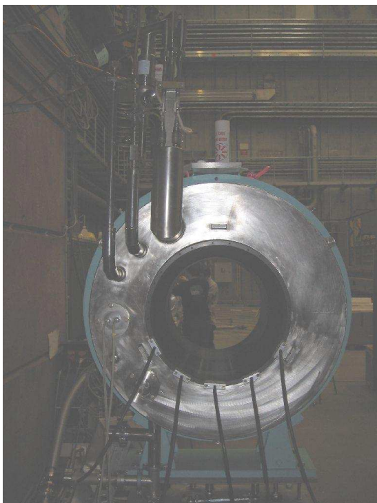
Figure 4.6: Cryostat in the test area, from left to right are visible the transfer line column, the bypass one and the thermal shield-current leads one. The service flanges are also visible with the connections for the temperature probes and the helium level probe. In the bottom left part of the cryostat the vacuum connection is placed.
