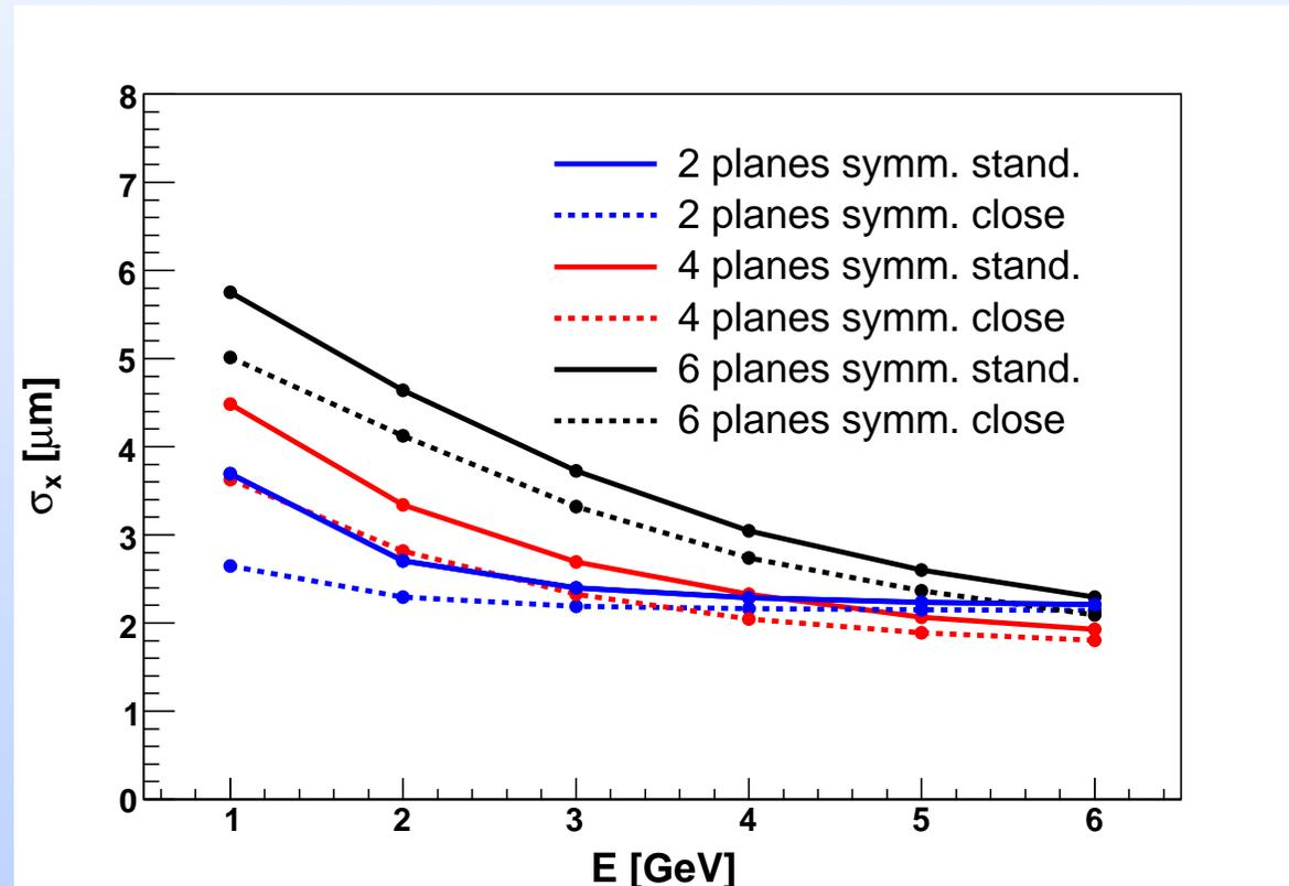
⇒ Telescope planes should be put as close as possible to the DUT
