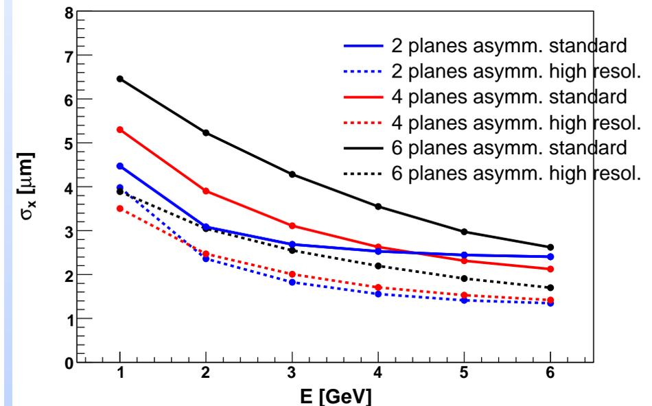
**In both cases the configurations with high density sensors for closest telescope planes give the best results**
