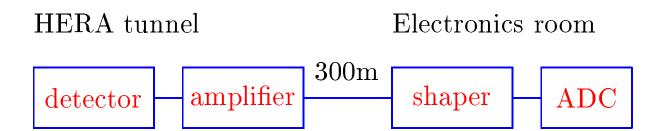
It might be necessary to have additional cable connections from the detector to the electronics (due to increased functionality of the electronics in the tunnel)
