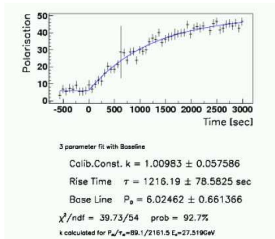
Example: risetime-curve (spin-rotators on) from end-of-fill summer 2006 → 40 mA in flat machine
