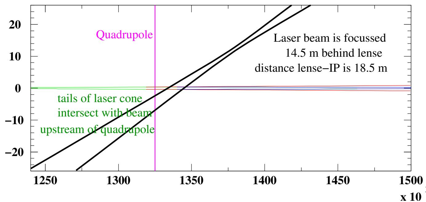
Conclusion: Compton beam has contribution from interactions downstream of Quadrupole
