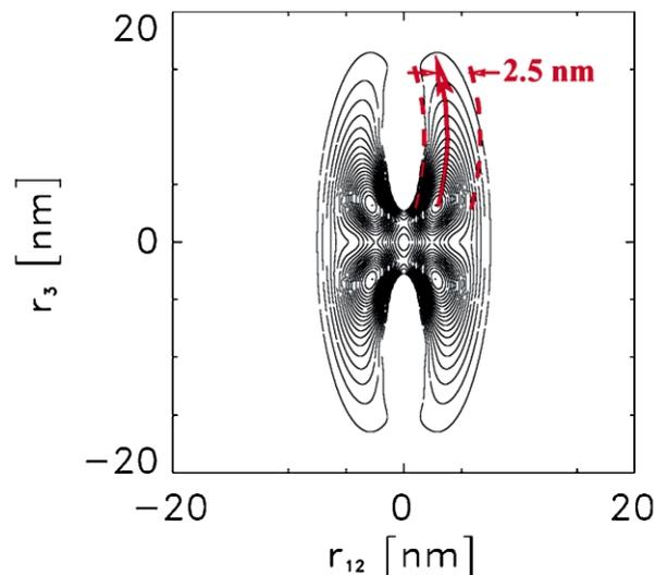
Fig. 13. Ultimate nanostructure of the polymer matrix of Nafion<sup>®</sup> 117. Positive contours of the domain peaks from the CDF. Strained state at  $\varepsilon = 1.25$ . The arrow indicates the correlation between domain height and orientation, starting from short and poorly parallelized domains. Broken lines indicate the estimation of the almost constant domain diameters.
