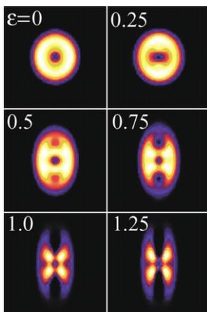
Fig. 9. Nanostructure of the polymer matrix of Nafion® 117 during elongation (transverse to MD). CDFs  $z(r_{12}, r_3)$ ,  $-20 \text{ nm} \leq r_{12}, r_3 \leq 20 \text{ nm}$ , (domain peaks) as a function of elongation  $\epsilon$ .
