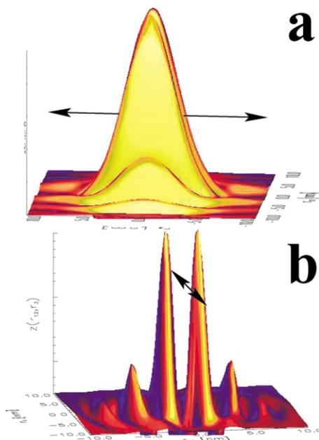
Fig. 5. Nafion 117<sup>®</sup> at  $\epsilon = 1.25$ . Domain dimension peaks from the CDF  $z(r_{12}, r_3)$  viewed (a) perpendicular and (b) parallel to the straining direction,  $r_3$ , indicated by double head arrows.
