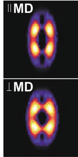
Fig. 10. Different straining directions and the nanostructure of Nafion 117. The CDF domain peaks are shown at  $\epsilon = 1.0$ . Straining direction is vertical. Narrow peaks (top) when straining in MD. Broader domain peaks (bottom) when straining in TD. Peak positions are identical.
