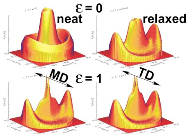
Fig. 1. Dry Nafion<sup>®</sup> 117 film. SAXS intensity  $I(s_{12}, s_3)$ , ( $-0.4 \text{ nm}^{-1} \leq s_{12}, s_3 \leq 0.4 \text{ nm}^{-1}$ ; long sample-to-detector distance) before, during and after straining to  $\varepsilon = 1$ . Bottom left: Strained in machine direction (MD). Bottom right: strained in transverse direction (TD).
