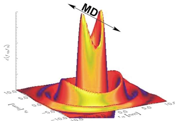
Fig. 3. Multidimensional chord distribution function (CDF)  $z_M(r_{12}, r_3)$  of the MAXS structure, ( $-10 \text{ nm} \leq r_{12}, r_3 \leq 10 \text{ nm}$ ) of Nafion 117<sup>®</sup> as extruded (domain peaks). Machine direction (MD,  $r_3$ ) is indicated by an arrow.
