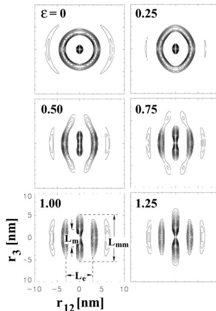
Fig. 6. Strained Nafion 117<sup>®</sup>. Contours of the negative peaks (related to the long periods) in the CDF of the MAXS structure. Straining direction ( $r_3$ ) is vertical.  $L_m$ : Most probable long period in meridional direction.  $L_{mm}$ : Maximum long period in meridional direction.  $L_e$ : Average long period in equatorial direction.
