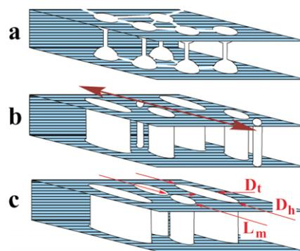
Fig. 8. Sketch of a void-layer structure and its evolution during straining of Nafion 117<sup>®</sup> that is compatible with the nanostructure data extracted from the measured MAXS patterns. (a) native material. (b) medium elongation. The straining direction is indicated by a double arrow. (c) high elongation. The domain thickness,  $D_t$ , domain height,  $D_h$ , and the meridional long period of the CDF,  $L_m$ , that is resulting from struts crossing the void-layers.
