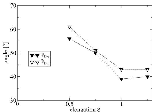
Fig. 12. Domain orientation of the matrix-related nanostructure of Nafion 117<sup>®</sup> in strained (filled symbols) and relaxed state (open symbols) as evaluated from the CDFs.  $\varphi_D$  is the most probable angle enclosed by the straining direction and the axis of the cylindrical domains.
