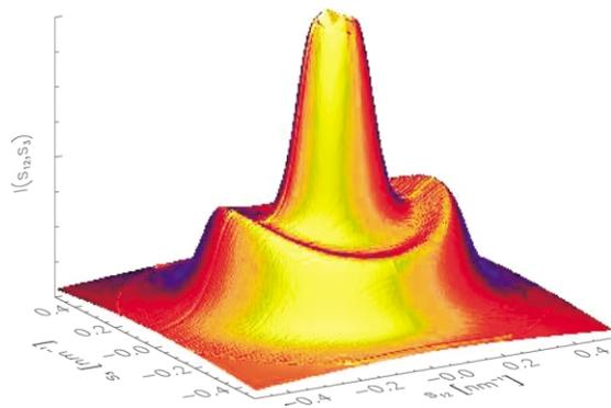
Fig. 2. Neat Nafion<sup>®</sup> 117. Scattering intensity  $\{I\}_2(s_{12}, s_3)$  projected onto the representative plane with the fiber axis chosen in MD. Visible range:  $-0.5 \text{ nm}^{-1} \leq s_{12}, s_3 \leq 0.5 \text{ nm}^{-1}$ .
