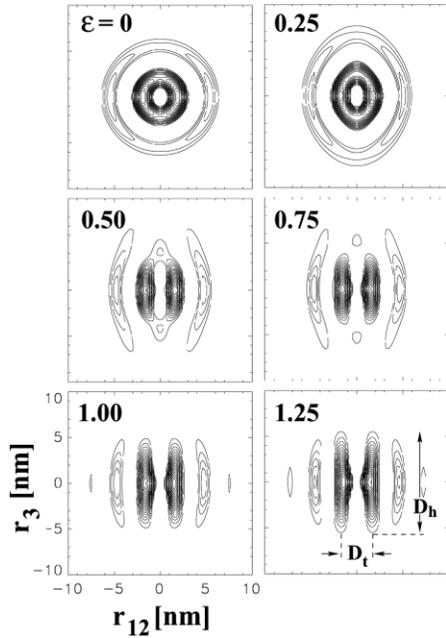
Fig. 4. Strained Nafion<sup>®</sup> 117. Contours of the positive peaks (related to the domains) in the CDF  $z_M(r_{12}, r_3)$  of the MAXS structure. Straining direction ( $r_3$ ) is vertical.  $D_t$ : Average domain thickness.  $D_h$ : Maximum domain height
