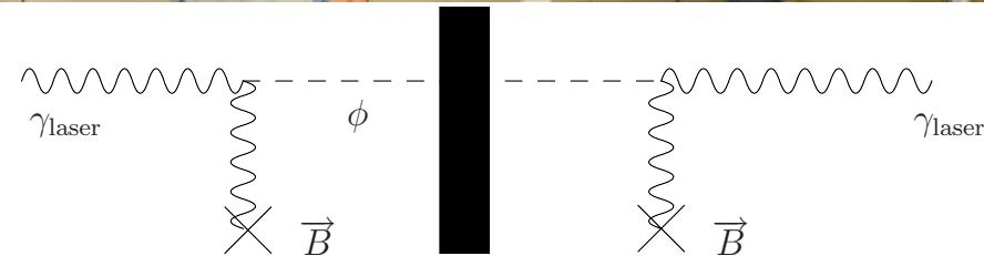
$$P(\gamma \rightarrow \phi) = P(\phi \rightarrow \gamma) = 4 \frac{(g\omega B)^2}{m_\phi^4} \sin^2 \left( \frac{m_\phi^2}{4\omega} L_B \right)$$
