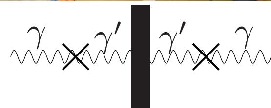
$$P(\gamma \leftrightarrow \gamma') = 4\chi^2 \sin^2 \left( \frac{L}{L_{\text{osc}}} \right); \quad L_{\text{osc}} = \frac{4\omega}{m_{\gamma'}^2} = 0.79 \text{ m} \left( \frac{\omega}{\text{eV}} \right) \left( \frac{\text{meV}}{m_{\gamma'}} \right)^2$$
