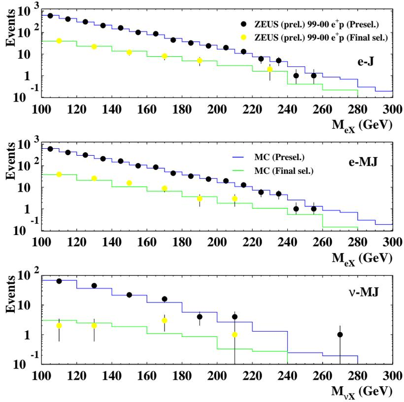
**Figure 3:** Comparison between data (dots) and SM MC (histograms) after pre-selection (dark dots and histograms) and final selection (light dots and histograms).
