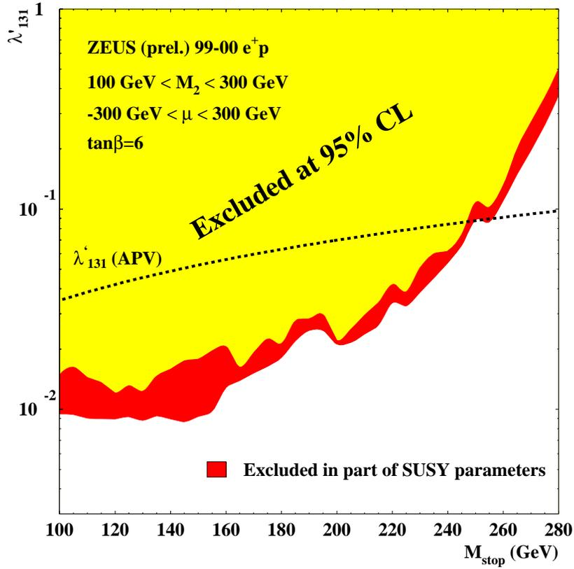
**Figure 4:** Limits on  $\lambda'_{131}$  as a function of the stop mass. The light (dark) region is excluded for all (part of the) considered SUSY scenarios. The limit from low-energy APV measurements is also shown.
