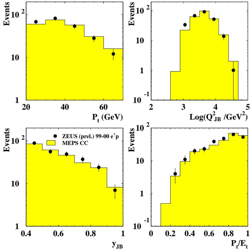
**Figure 2:** Comparison between data (dots) and SM MC (histograms) for  $P_t$ ,  $\log_{10}(Q_{JB}^2 / \text{GeV}^2)$ ,  $y_{JB}$  and  $P_t/E_t$ .
