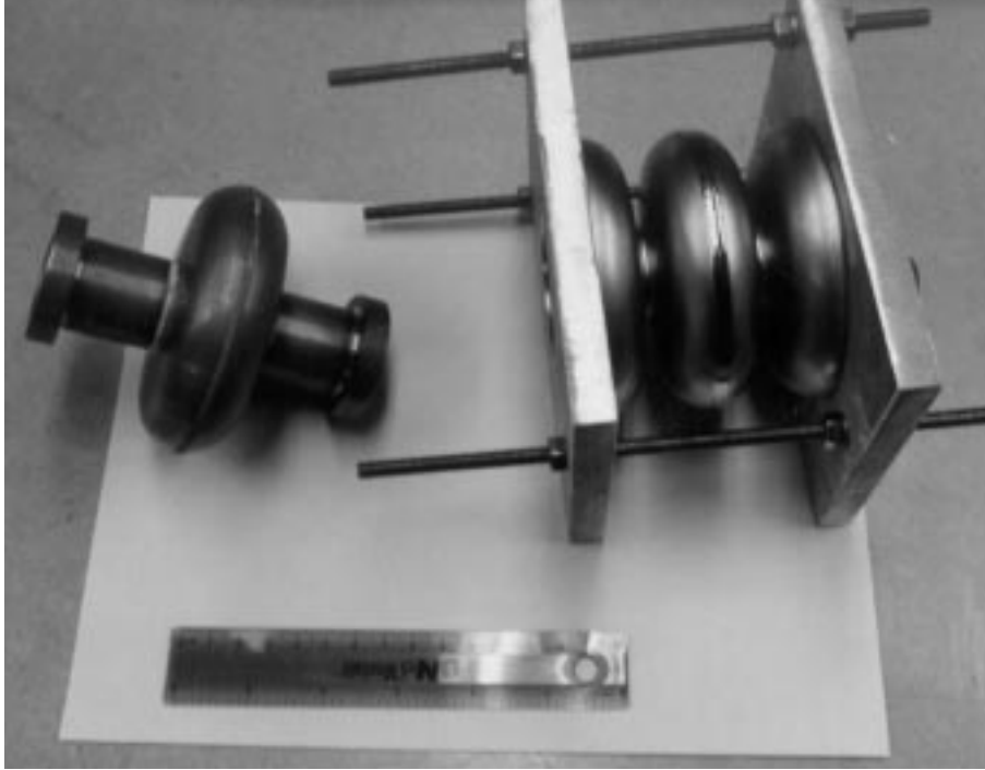
Figure 2: Copper and niobium models of the transverse mode cavities. Two shorting plates have been added to the one cell and two half cell niobium model.
