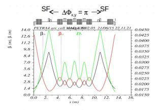
Figure 5: Conceptual layout of a six bend cell with a  $\pi$ -phase advance between sextupoles.
