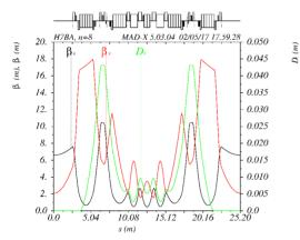
Figure 2: Hybrid seven bend achromat cell (length 25.5 m) with a bare cell emittance of 12 pm rad.
