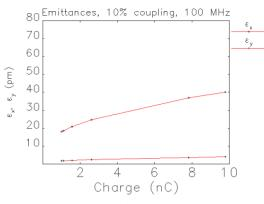
Figure 3: Emittance with IBS versus bunch current.
