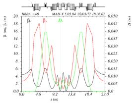
Figure 4: Hybrid six bend achromat cell (length 23 m) with a bare cell emittance of 25 pm rad.
