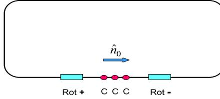
**FIGURE 2.** A schematic layout for the rotators (Rot $\pm$ ) and some TE cavities (C) for exploiting the longitudinal Stern-Gerlach effect.
