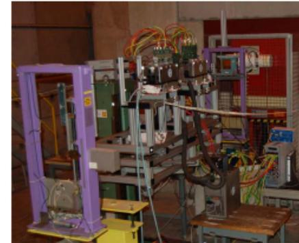
EUDET Telescope for test beam use.
