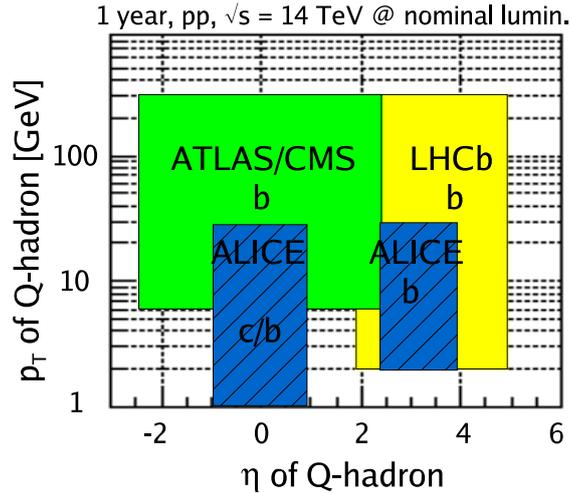
**Fig. 2:** Schematic acceptances in transverse momentum and pseudorapidity for open heavy flavour hadrons (indicated as ‘Q-hadrons’) in the four LHC experiments. The high- $p_T$  coverages correspond to one year (i.e. 7 months) of running at nominal luminosity (see beginning of this section).
