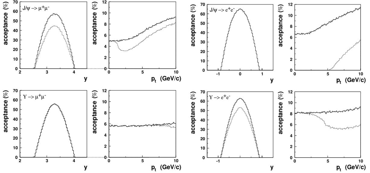
**Fig. 6:** Acceptance for  $J/\psi$  and  $\Upsilon$  as a function of  $y$  and  $p_T$  for measurements in the di-muon channel and di-electron channels. To give an idea of the effect of the trigger, the acceptances are shown without (solid) and with (dashed) a sharp cut on the transverse momentum of single muons of 1 GeV/c (2 GeV/c) for  $J/\psi$  ( $\Upsilon$ ) and for single electrons of 3 GeV.
