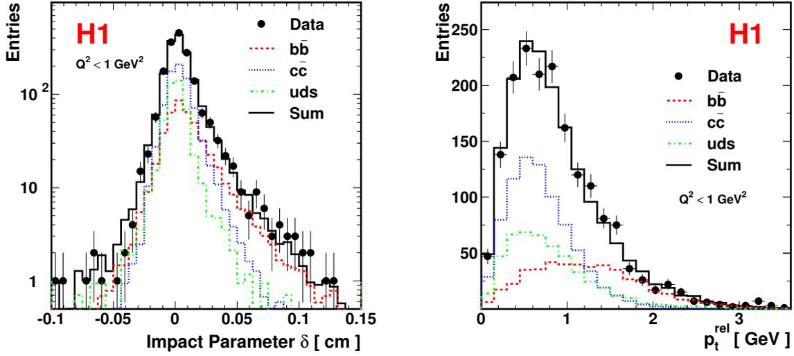
**Fig. 6:** Distributions of the impact parameter  $\delta$  of the muon track (left) and the transverse muon momentum  $p_t^{rel}$  relative to the axis of the associated jet (right) in H1. Also shown are the estimated contributions of events arising from  $b$  quarks (dashed line),  $c$  quarks (dotted line) and the light quarks (dash-dotted line).
