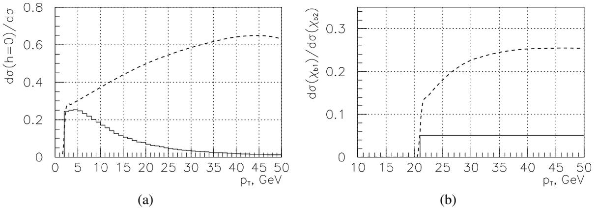
**Fig. 9:** Predictions of different theoretical approaches for quarkonium production. In (a) the fraction of longitudinally polarized  $\Upsilon$  mesons is shown: solid histogram – collinear parton model, singlet + octet; dashed –  $k_t$ -factorization with KMS u.g.d.. In (b) the ratio of the production rates  $\chi_{b1}/\chi_{b2}$  is shown: solid histogram – collinear parton model, singlet + octet; dashed –  $k_t$  factorization with KMS u.g.d.
