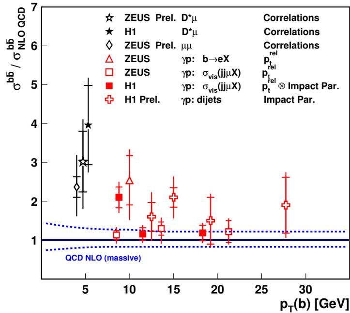
**Fig. 10:** Ratio of beauty production cross section measurements in photoproduction at HERA to NLO QCD predictions in the massive scheme as function of the transverse momentum of the  $b$  quark  $p_{Tb}$ . The dashed line gives an indication of the size of the theoretical uncertainties.
