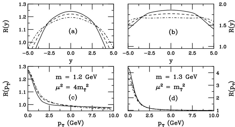
**Fig. 8:** We present  $R(y)$ , (a) and (c), and  $R(p_T)$ , (b) and (d), in  $pp$  collisions at  $\sqrt{S} = 14$  (solid), 8.8 (dashed) and 5.5 (dot-dashed) TeV. The left-hand side shows  $m = 1.2$  GeV and  $Q^2 = 4m_T^2$ , the right-hand side  $m = 1.3$  GeV and  $Q^2 = m_T^2$ .
