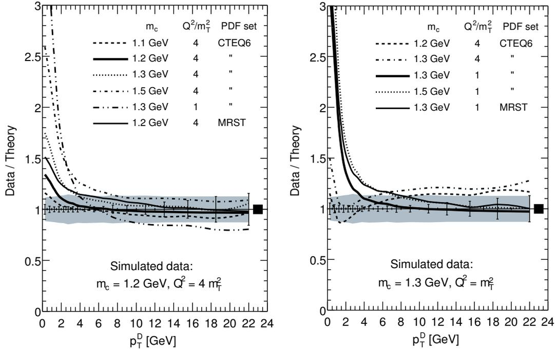
**Fig. 11:** Ratio of the generated ALICE data relative to calculations of the alternative NLO cross sections with several sets of parameters and PYTHIA string fragmentation. The left-hand side shows the result for  $m = 1.2$  GeV and  $Q^2 = 4m_T^2$  while the right-hand side is the result for  $m = 1.3$  GeV and  $Q^2 = m_T^2$ .
