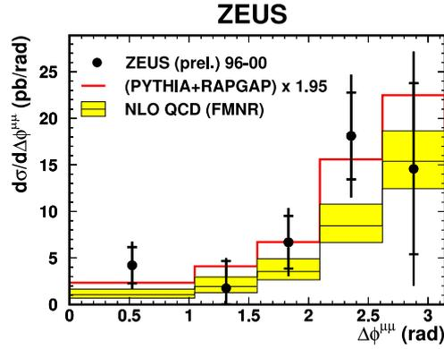
**Fig. 16:** Differential cross section  $d\sigma/d\Delta\phi^{\mu\mu}$  for dimuon events from  $b\bar{b}$  decays in which each muon originates from a different  $b(\bar{b})$  quark. The data (solid dots) are compared to the leading order + parton shower generators PYTHIA and RAPGAP (histogram) and to massive NLO QCD predictions (shaded band).
