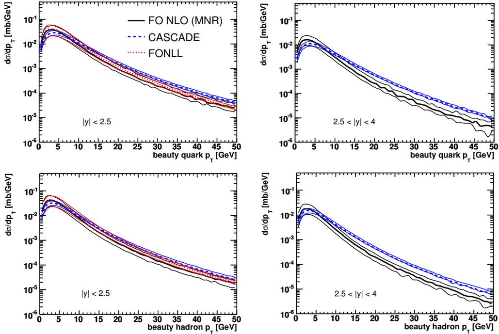
**Fig. 7:** Cross sections for beauty production in  $pp$  collisions at the LHC with  $\sqrt{s} = 14$  TeV. The differential cross sections in  $p_T$  for  $b$  quark in the two rapidity ranges  $|Y| < 2.5$  and  $2.5 < |Y| < 4$  are shown in the upper panels. The lower panels show the cross sections for the production of a beauty hadron as a function of  $p_T$  in the same rapidity ranges.
