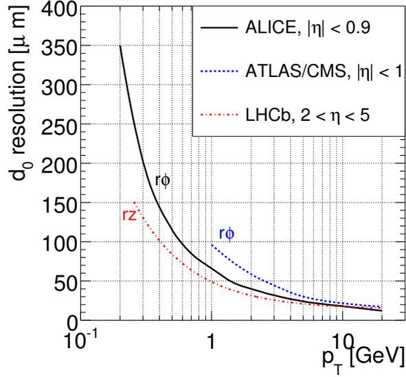
**Fig. 1:** Track impact parameter resolutions for the four LHC experiments. Note that for ALICE, ATLAS and CMS the impact parameter is defined in the  $r\phi$  plane, while for LHCb it is defined in the  $rz$  plane.
