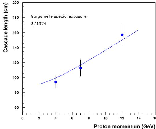
Figure 5: Measured and predicted proton cascade length versus proton momentum.
