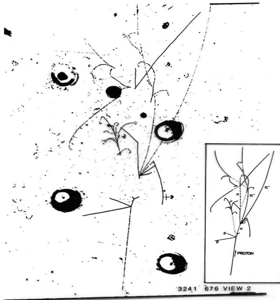
Figure 6: Proton cascade observed in Gargamelle. A 7 GeV proton enters from below and generates a cascade as interpreted in the inserted sketch.
