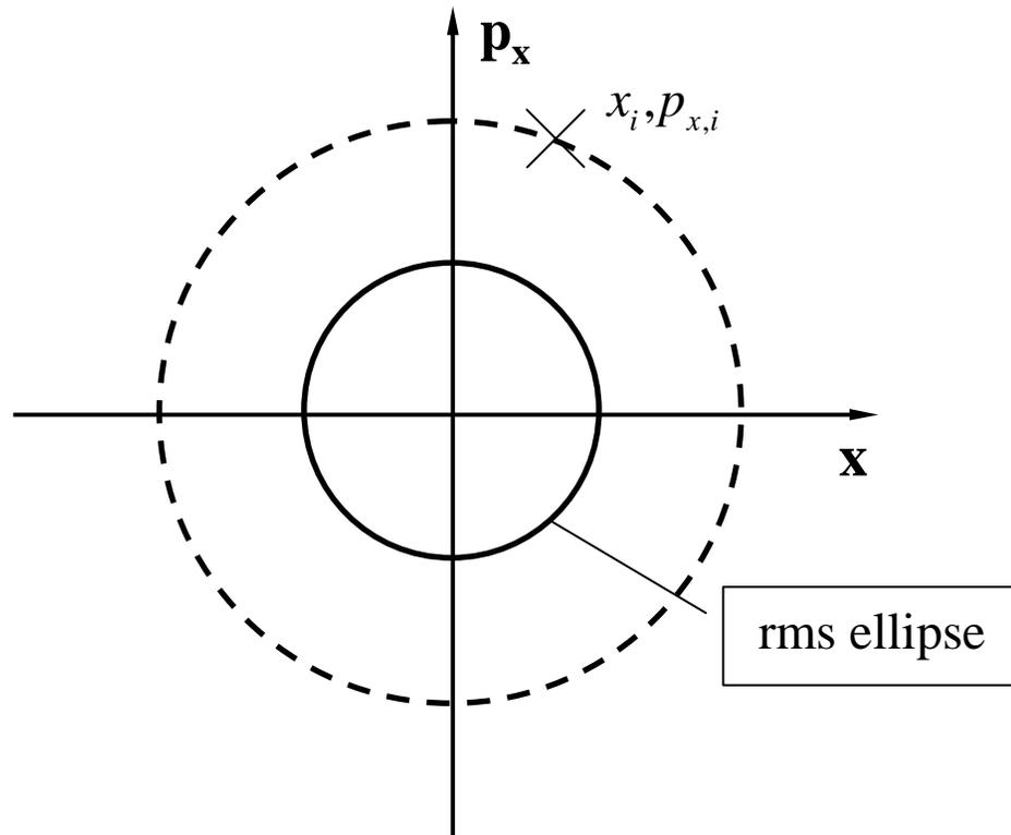
The rms ellipse of the beam is transformed into a circle.
