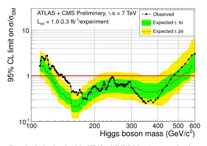
Figure 21: Combined results of the ATLAS and CMS Collaborations presented at the Hadron Collider Workshop in November 2011. The solid line is the experimental upper bound, at 95% confidence level, on the cross section for Higgs boson production divided by the cross section of the Standard Model. The dashed line is the expected 95% exclusion bound, and the green and yellow bands are the one- and two-standard deviation bands around that expected bound.
