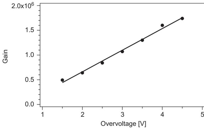
Fig. 6. SiPM gain as a function of the overvoltage.
