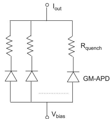
Fig. 2. The equivalent circuit of the SiPM.
