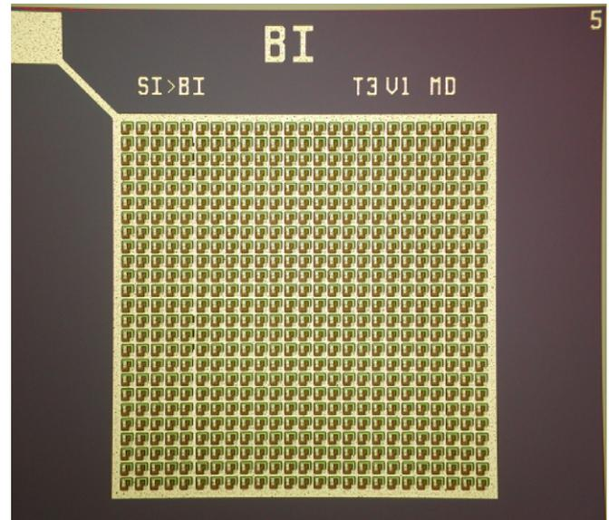
Fig. 1. Photograph of a SiPM prototype from ITC-irst.
