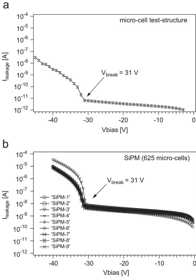
Fig. 3.  $I$ - $V$  reverse characteristics of (a) single micro-cell test structure and (b) nine SiPM devices each with 625 micro-cells.
