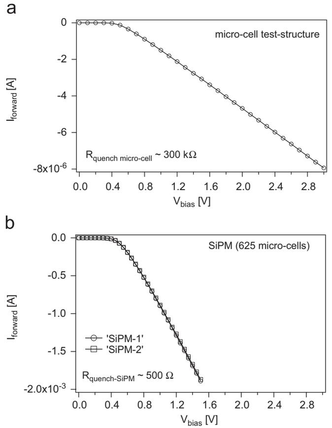
Fig. 4.  $I$ - $V$  forward characteristics of (a) a single micro-cell test structure and (b) two SiPM devices.
