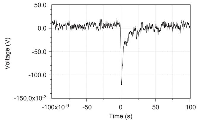
Fig. 5. Dark pulse from a SiPM micro-cell at 4 V over  $V_{break}$ .
