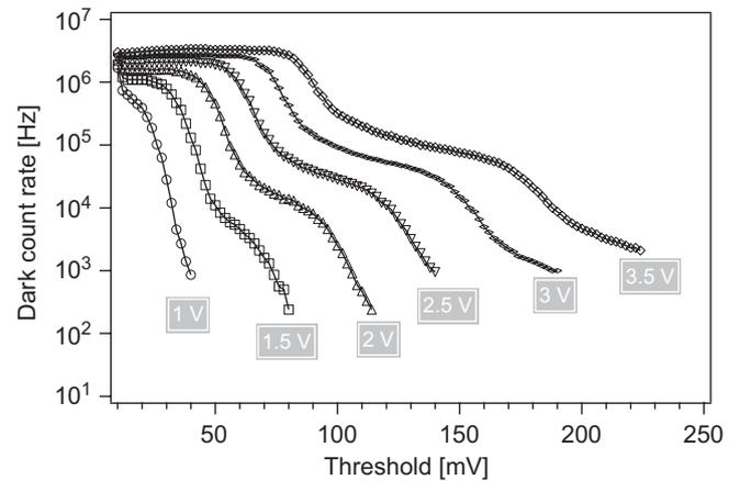
Fig. 7. SiPM dark count rate as a function of pulse amplitude (threshold) for different overvoltages.
