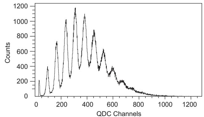
Fig. 8. SiPM single photoelectron spectrum measured with a pulsed low-light-level LED at 33.5 V.
