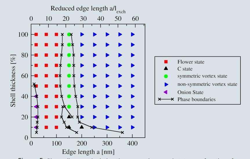
Figure 5: Phase diagram depicting the energetic ground state as a function of the two parameters a and  $t_{rel}$ . The shell thickness is varied between the limits of a infinitely thin shell and a solid pyramid. The ground state is the configuration with the lowest energy and, as such, is a stable configuration.
