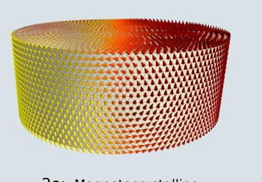
2e: Magnetocrystalline anisotropy - the lattice structure of material influences the magnetic configuration. Here we "switched on" a linear anisotropy in z direction.
