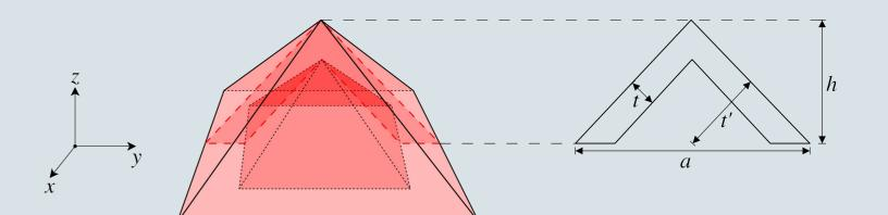
Figure 3: Sketch of the studied geometry. We consider two parameter: the side length a of the basal plane determines the size of our geometry. The relative thickness  $t_{rel} = 100.0 \cdot t / t'$  is a shape parameter. The height h is set to a/2. The magnetic properties of the core are assumed to be negligible, so that only the shell is considered by the model.
