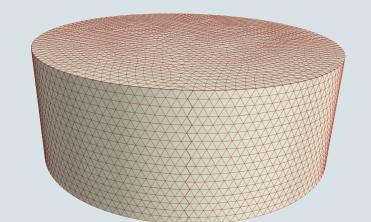
Fig.2a: Finite number of degrees of freedom by discretising fields on an unstructured mesh (finite element method)
