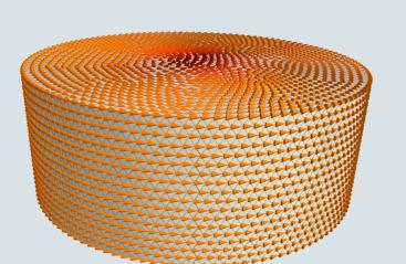
2d: Magnetostatic interaction of magnetisation. Magnetisation at the surface tries to align parallel to surface. As in our example, this interaction often leads to the formation of vortices.
