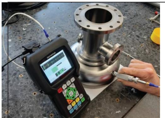
Figure 3: Ultrasonic wall thickness measurement device.
