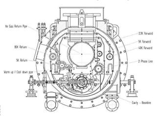
Figure 4: The cryomodule transverse cross-section.
