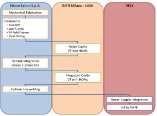
Figure 2: Cavity production and test workflow.
