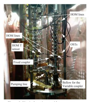
Figure 1: Vertical test insert with two prototypes.
