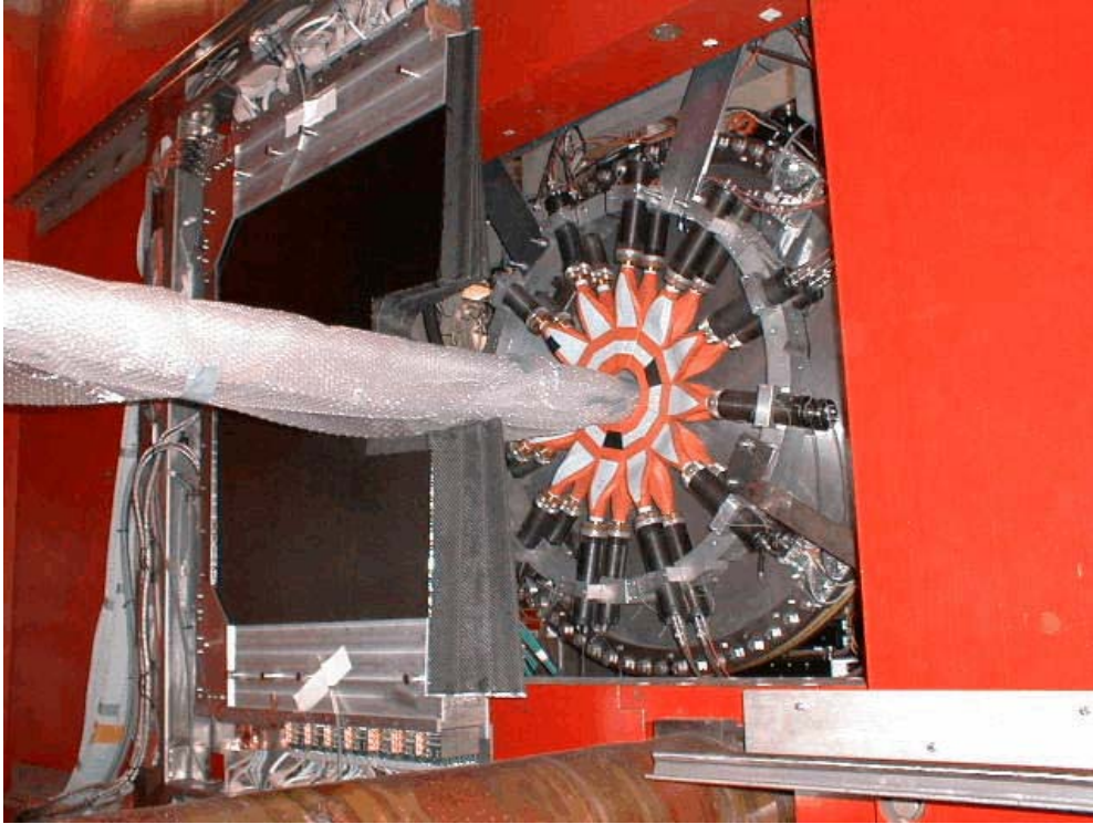
Fig. 9. HERA-B Trigger Ring - 12 scintillation hodoscopes fixed at the exit window of the VDS vessel to monitor the overall interaction rate and/or the individual target contribution by the asymmetry method [8,25].
