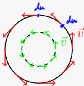
$$\begin{aligned} E_{\text{kin}} &= \sum_i \frac{1}{2} m_i v_i^2 \rightarrow \int \frac{1}{2} v^2(\rho) d m \\ &= \frac{1}{2} \int \omega^2 r^2 d m = \frac{1}{2} \omega \underbrace{\int r^2 d m}_I \end{aligned}$$
