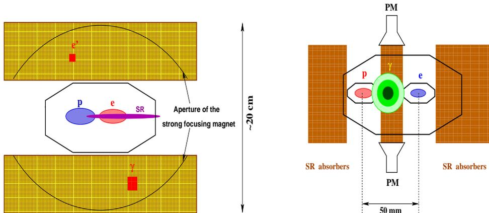
Figure 1: Options for the luminosity monitoring. (a) QEDC tagger at  $z = -6\text{m}$ ; (b) active SR absorber and luminosity detector at  $z = -22\text{m}$ .
