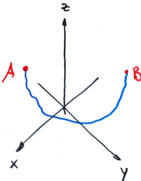
$$\vec{r}(t) = \begin{pmatrix} x(t) \\ y(t) \\ z(t) \end{pmatrix} = x(t)\vec{e}_x + y(t)\vec{e}_y + z(t)\vec{e}_z$$
