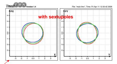
Phase space portraits of monochromatic 3o ellipses (matched at the entrance) after tracking through the extraction arc. The relative energy deviations are equal to -1.5%, 0% and + 1.5% (red, green and blue ellipses, respectively).
