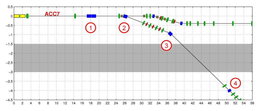
Two kickers. Each 1 *m* long with maximal field 0.005 *T*. This gives  $\sim$ 2 *mrad* beam deflection and  $\sim$ 13 *mm* beam offset from the linac axis at the septum entrance.
