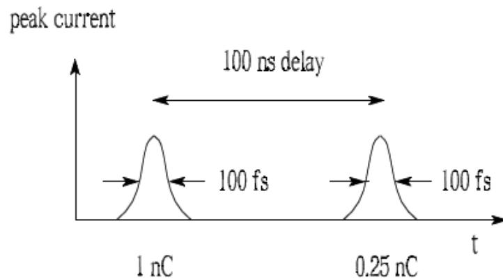
Fig. 26. Double electron bunch generation for THz pump/X-ray probe experiments at the LCLS. The THz radiation transport through the access maze introduces a path delay with respect to the X-ray path, which has to be compensated with the introduction of a delay between two bunches.
