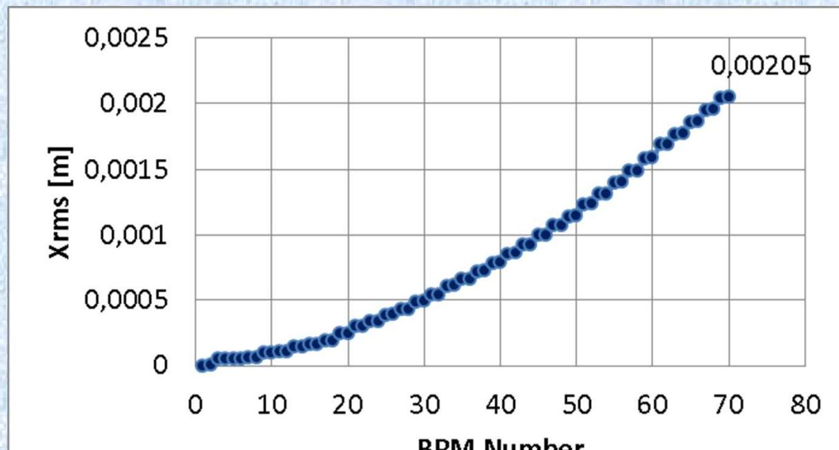
Doubling the quantity of BPMs leads to the reduction of  $X_{\text{rms}}$  by a factor of about  $\sqrt{2}$ .
