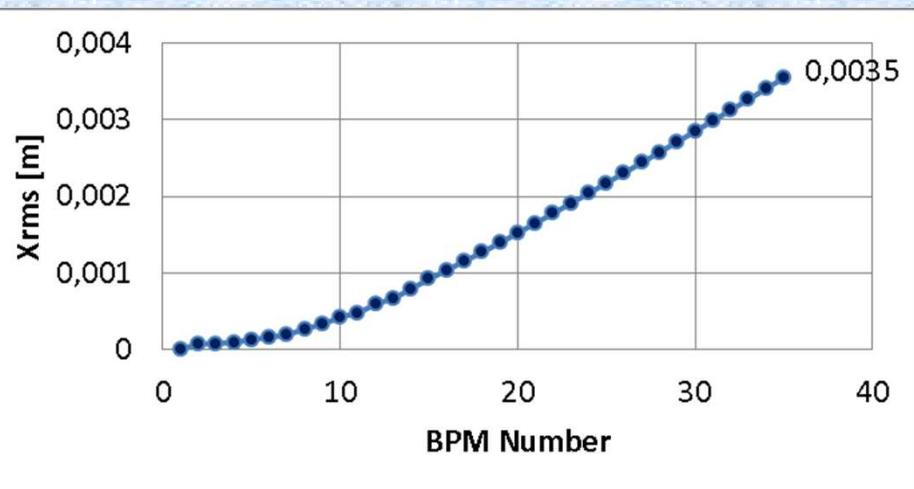
Only the first half of BPMs has 1 $\mu$ m rms resolution errors
