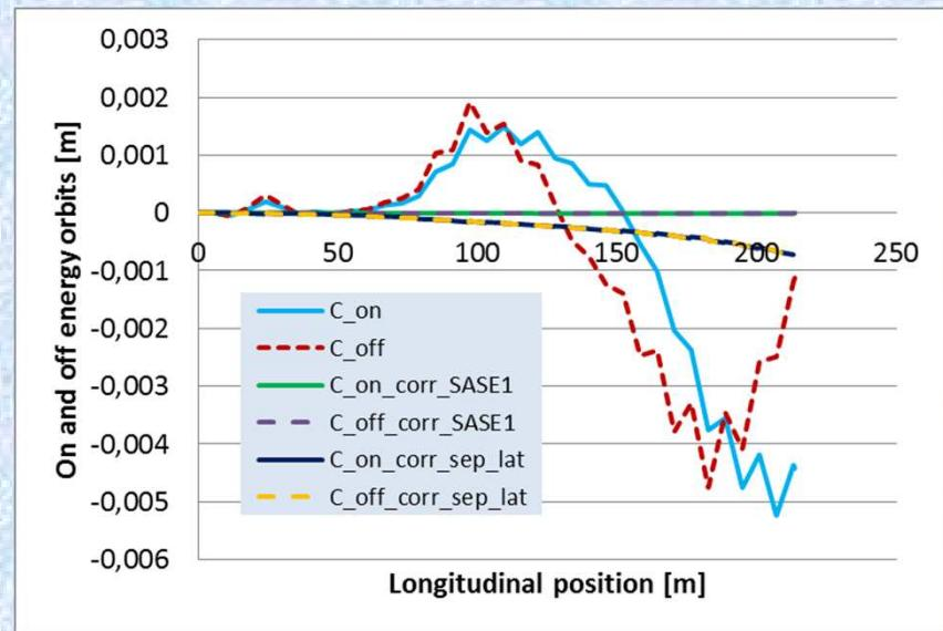
Comparison of rms residual orbits for SASE1 and separated elements lattices for  $\sigma_{\text{res}} = 1\mu\text{m}$ ,  $\delta = -0.4$ .
