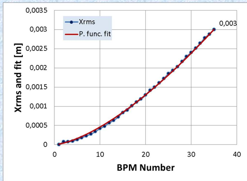
$X_{rms}$  and power function fit  $a^*n^b$  for SASE1 for  $\sigma_{res} = 1 \mu\text{m}$ ,  $\delta = -0.02$ ,  $\mu = 0.4\text{rad}$ .
