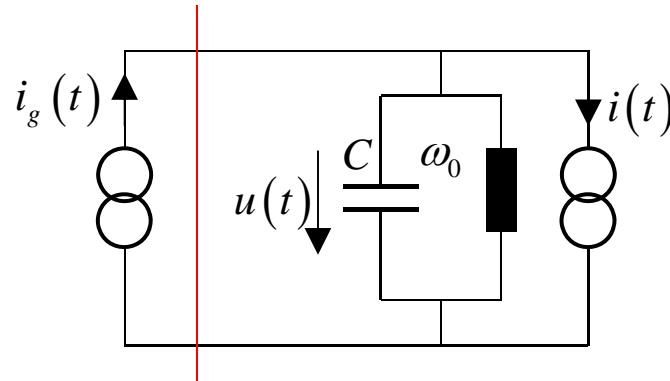
calculate the generator current with help of an external network
