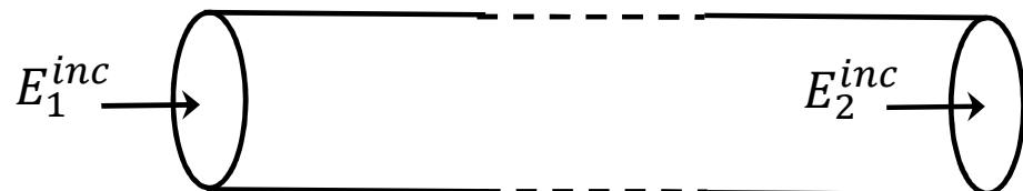
2D-electrostatic problem at both ends of the pipe
