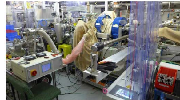
Gun4.5 installation into the PITZ beamline and baking of the gun system
