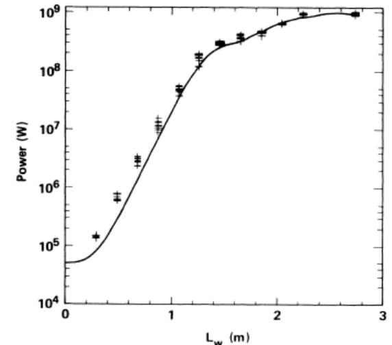
FIG. 3. Amplified signal output as a function of wiggler length for tapered wiggler field. Crosses indicate experimental values and the solid line is the results of the numerical evaluation.
