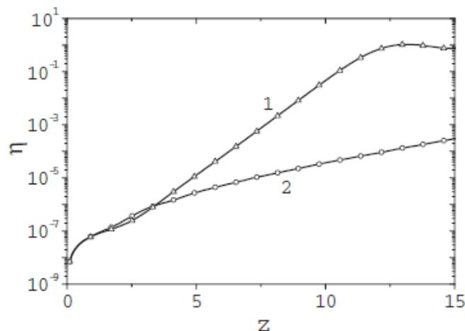
FIG. 3. Normalized power versus undulator length. Solid line 1:  $\hat{\alpha} = 0$ ,  $\hat{b}_1 = 0$ ; triangles:  $\hat{\alpha} = 4$ ,  $\hat{b}_1 = -2$ ; solid line 2:  $\hat{\alpha} = 4$ ,  $\hat{b}_1 = 0$ ; circles:  $\hat{\alpha} = 0$ ,  $\hat{b}_1 = 2$ .
