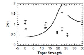
Fig. 2. The experimental normalized efficiency  $2N\eta$  vs. taper strength is shown. The curve is scaled from the one in Ref. [8]. The circles are CW efficiencies, the diamonds are pulsed efficiency and the triangles are the pulsed efficiency for the case of  $Q = 50$ . The filled symbols are taken at  $3 \mu\text{m}$  and the empty ones at  $6 \mu\text{m}$ . Two of the symbols are slightly offset at  $b = 0$  for clarity.
