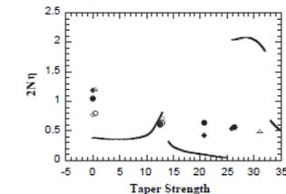
Fig. 3. The experimental normalized efficiency vs. taper strength for a positive taper is shown. The curve is scaled from Ref. [8]. The symbol definition is the same as for Fig. 2.
