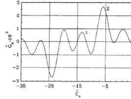
Fig. 2. The reduced small-signal gain versus the reduced detuning at the undulator entrance. Here  $b = 30$ . (1) – the first maximum, (2) – the second maximum.
