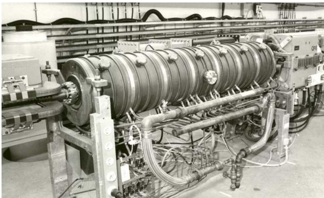
input coupler waveguide transition,
