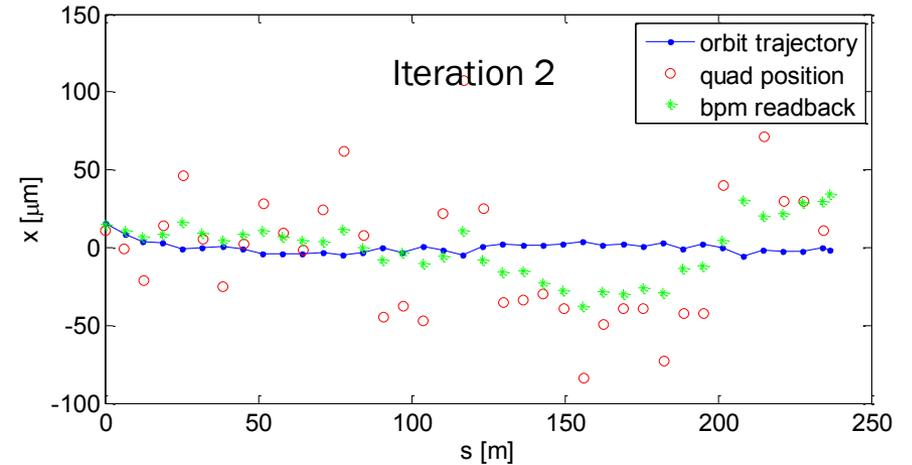
$\langle x \rangle_{rms}=0.7\mu m, \langle x_{BPM} \rangle_{rms}=4.3\mu m, \langle x_{QUAD} \rangle_{rms}=7.8\mu m$
