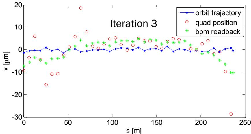
Orbit trajectory (blue line), quadrupole position (red circle), and BPM readback (green star) for 1 random seed during 3 iterations at 17.5 GeV (linear component removed for clarity).
