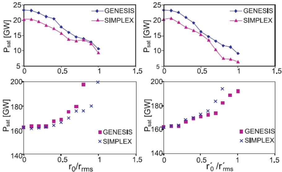
Figure 3: Saturation power (top) and saturation length (bottom) versus beam initial space (left) and angular (right) offsets.
