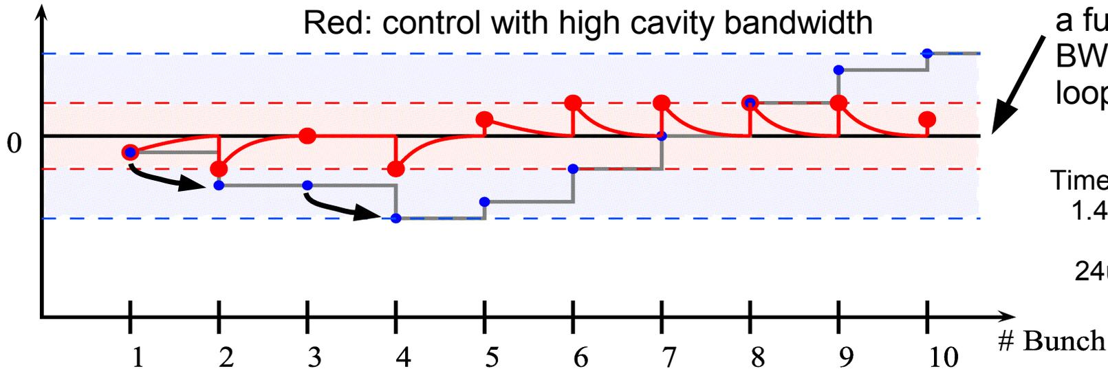
Max. error is a function of BW (and loop delay)
