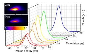
FIG. 2. Experimental scattering spectra as function of time delay. The inset shows two 16-bit raw spectra, each  $25 \times 50$  pixels of  $(13.5 \ \mu\text{m})^2$  size, with a horizontally oriented spectral axis corresponding to the graph, where the spectral profiles are integrated along the vertical axis.
