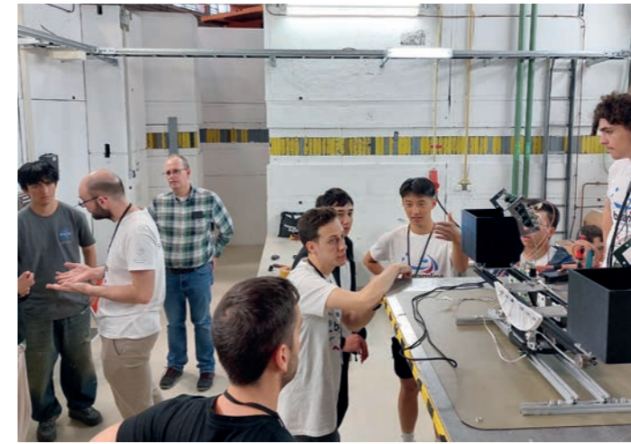
Figure 2 Setup of the experiments at Beamline T21. The muon detector setup of the team Dawson Technicolor, including the rotatable support structure, can be seen at the bottom right.
