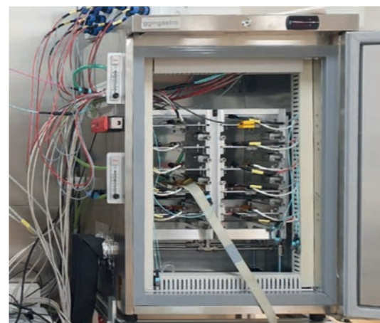
Figure 2 Burn-in test setup with modules to be tested on the support structure inside the refrigerator. The second setup is identical.
