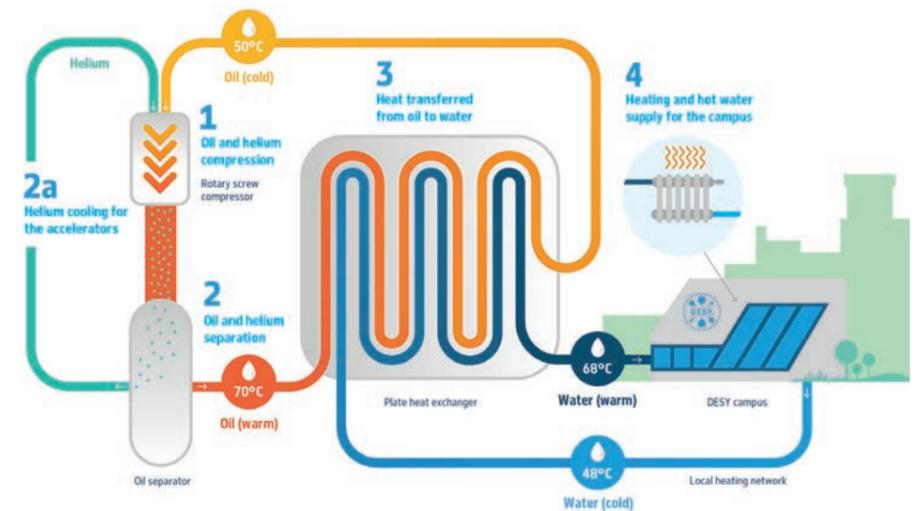
Waste heat recycling system at DESY: The accelerators and their support systems can be used to warm the entire campus. So far, a third of the campus is heated in this way.
