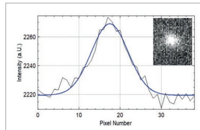
**Figure 2** Left: Beam profile at the detector corresponding to an accumulated 30  $\mu$ m aperture raster scan of the beam at the target position. Right: Profile of the streaked electron beam at optimal compression phase. Insets: Image of the streak camera and recorded streak image.
