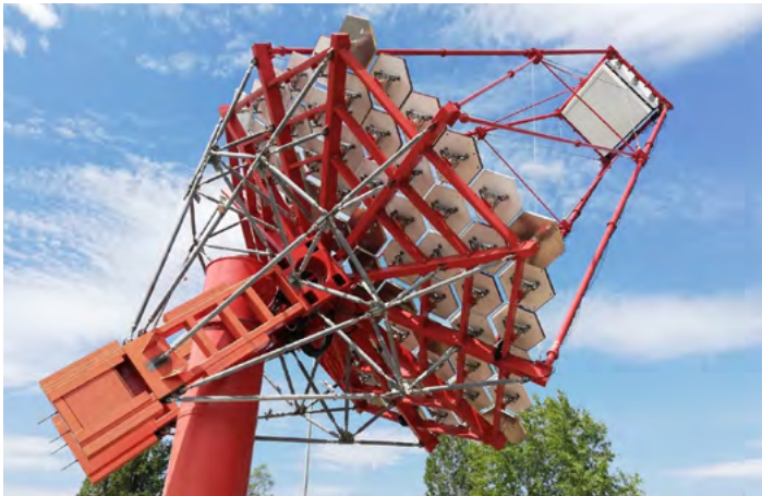
Figure 2 MST prototype structure in Berlin-Adlershof equipped with the Cherenkov camera NectarCAM (May 2019)
