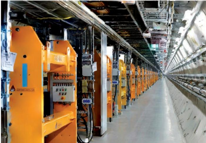
The undulators of the SASE3 beamline, the second X-ray light source to take up operation at the European XFEL X-ray laser
