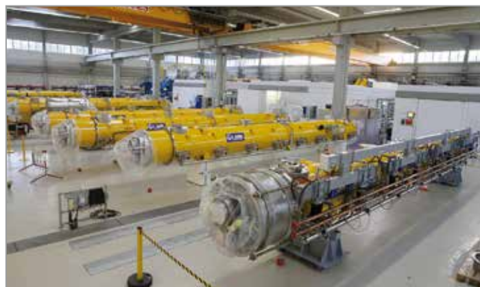
Figure 1 Accelerator cryomodules in the AMTF in front of the test stands
