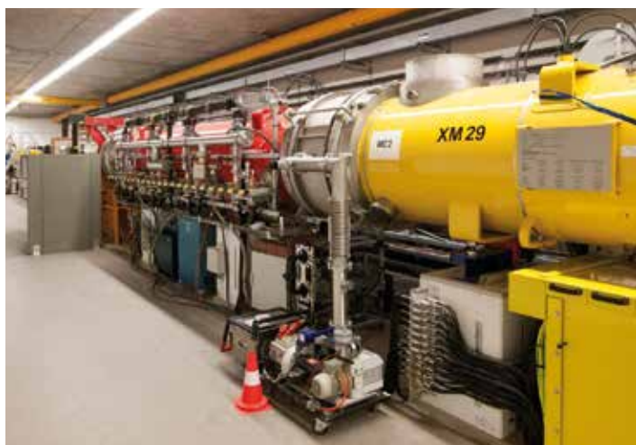
The 30 m long injector of the European XFEL
