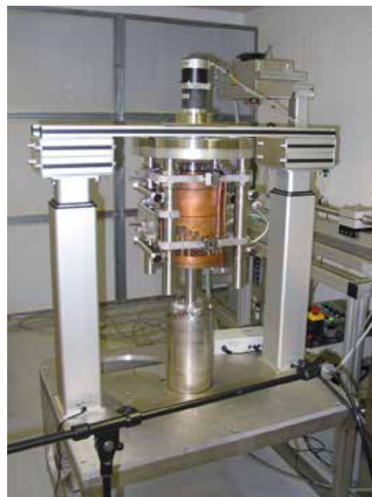
Figure 1 Dry-ice cleaning device for RF guns at DESY, with a 1.3 GHz gun installed
