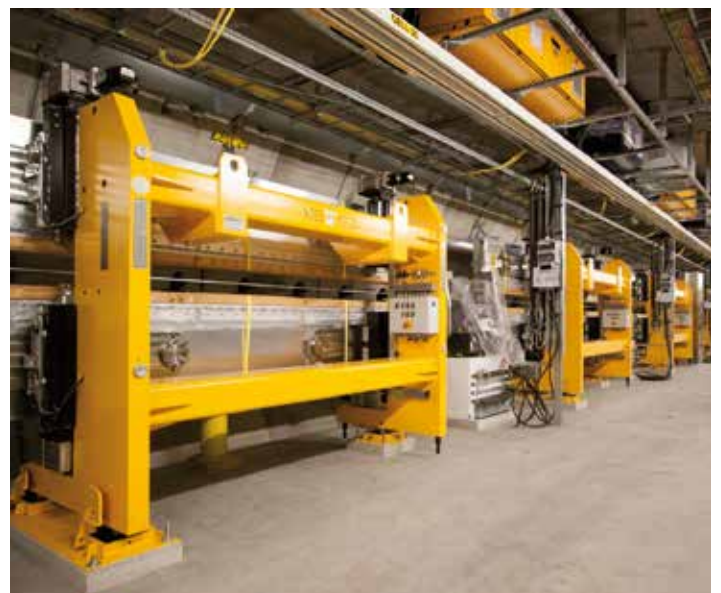
The first undulator of the European XFEL consists of 35 segments, each 5 m long and weighing 7.5 t.
